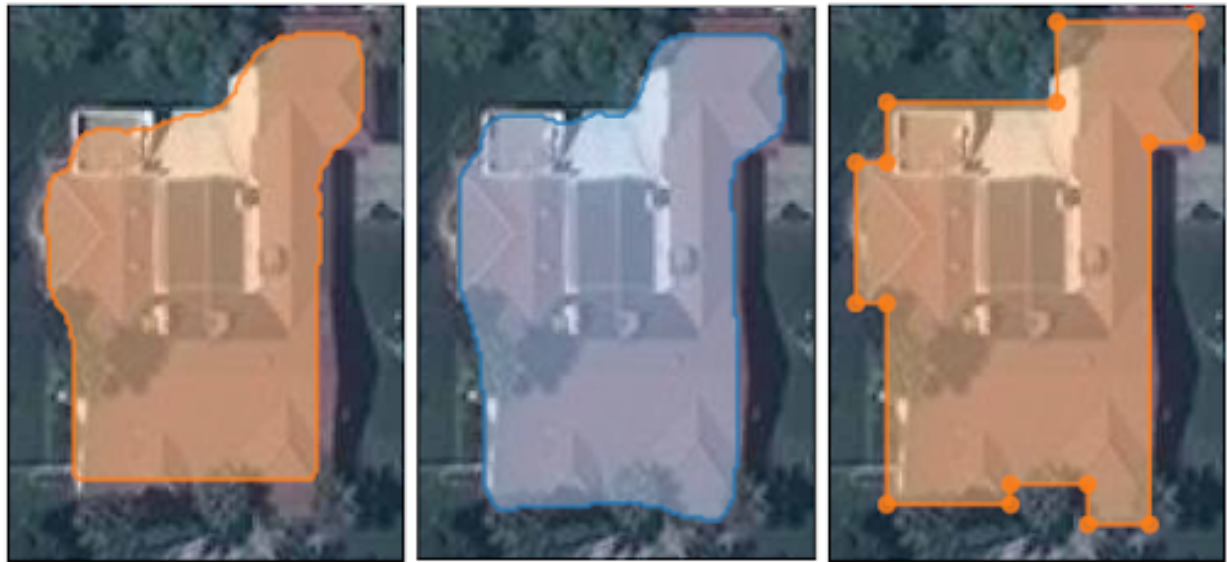
Figure 8: A comparison of polygons generated by instance segmentation (left) and PolyMapper, which uses fewer vertices and preserves right angles (right) , source
